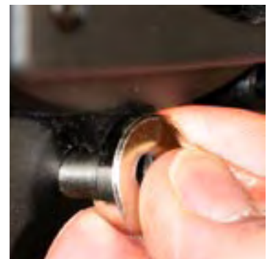
1) Grasp the Emergency Eject Knob
